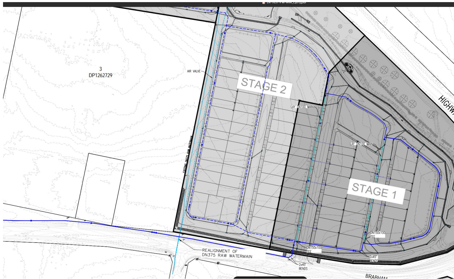
1 Raw Waterline to be relocated under parking lane
